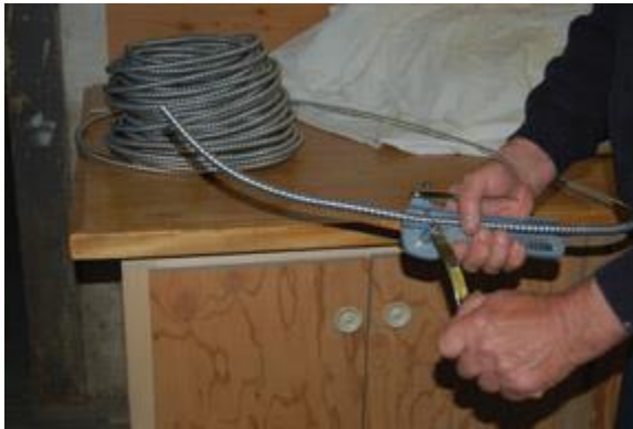
Photo 1. The only specialized tool needed to work with MC cable is an MC cutter. Two or three turns of the handle, and the metal sheath is cleanly severed without compromising the enclosed conductors.
